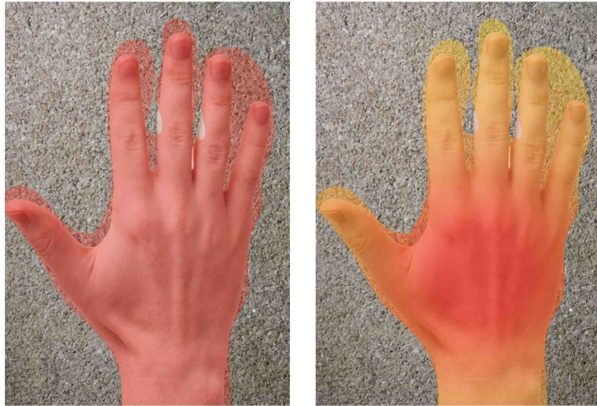
Fig. 4. On the left: a simplified representation of the original Crayons interface, which shows classification of an image based on a binary threshold. On the right, a confidence-based visualisation which exposes how the classifier may still be uncertain about the fingers, and thus additional annotation may be beneficial.
